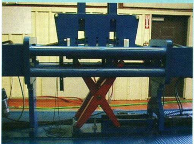
Fig. 9. CTTM Bending Fixture — Sample Bent
