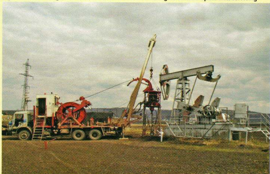
Fig. 2. Coiled tubing unit M1002 with 25.4 mm O.D. tubing for annular space well servicing
