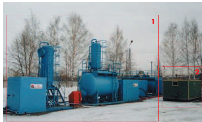
Fig. 3 Closed-type Circulation System and Pump Block
