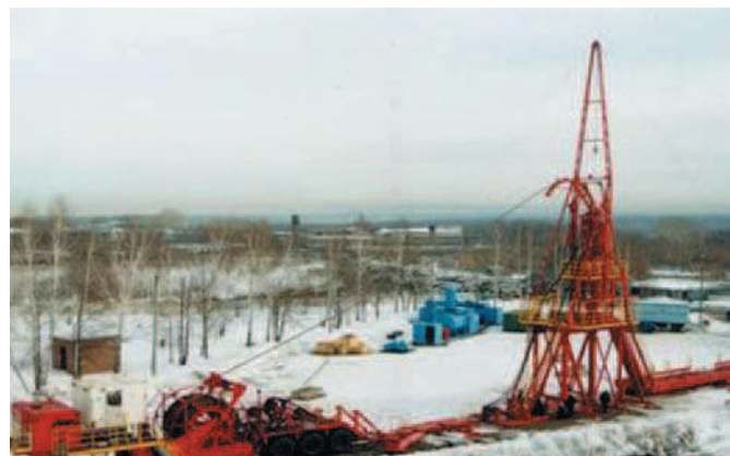
Fig. 2. Underbalanced Drilling System with Coil Tubing Aggregate Applied
