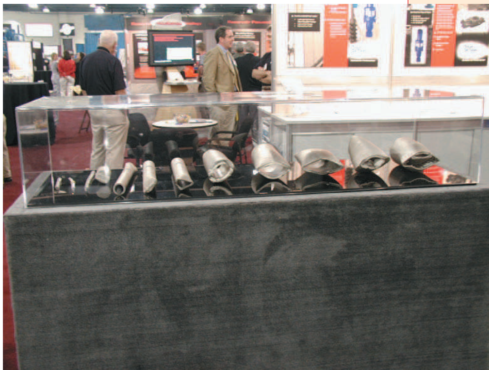
▲ CT characteristics after shear rams' work of the preventers of «Texas Oil Tools»
