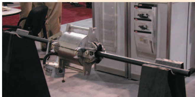
CTES device to control geometry of CT
