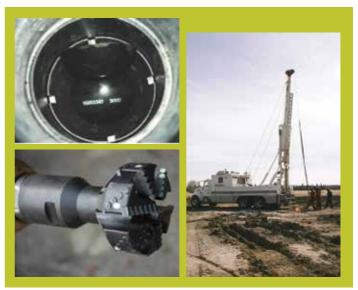
switched to high RPM to allow for ball drilling out. The ball and the seat No 3 were milled out in 15 min. During the next 3 minutes a half of the ball was milled out at low RPM and it took 27 minutes to mil out the ball of the forth seat. Seat No 5 itself did not have to be milled as it isolated the bottomhole, which was not needed for access.
