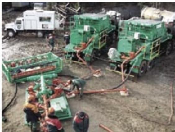
power. Depending on the chosen plunger diameter the output of the pump can reach 1510 gal/min. The working pressure of the pumping unit is up to 19870 PSI.
