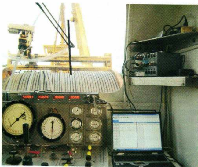
Fig. 4. Typical data acquisition system consists of data collection unit, displays, sensors, cables, computer and software.
