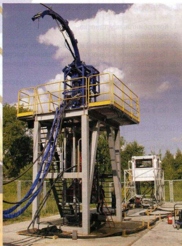
Pictures: injector with 24 ton lifting capacity on the test bench Photos permitted by CJSC FIDMash
