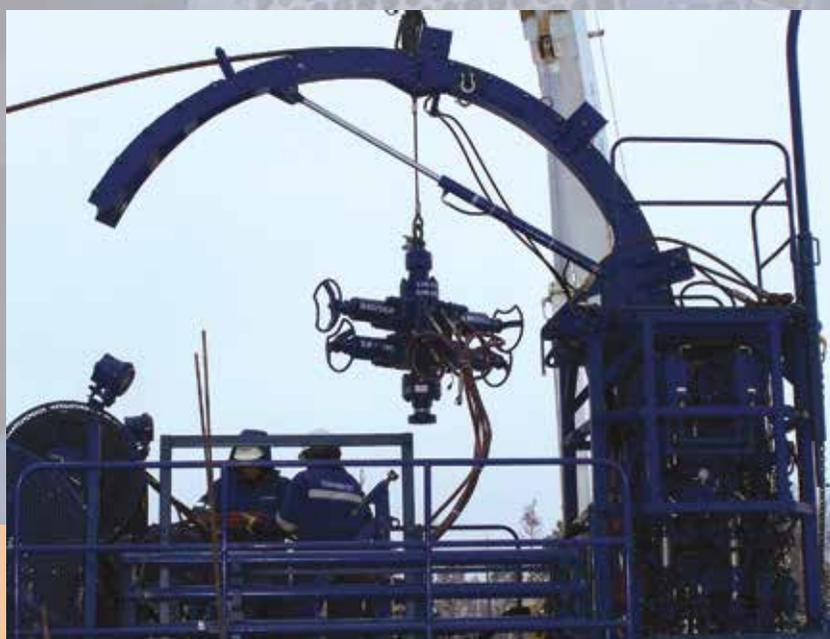
Pictures: injector with 24 ton lifting capacity on the test bench
