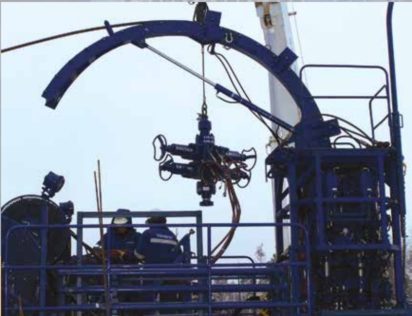
Pictures: injector with 24 ton lifting capacity on the test bench Photos permitted by NOV Fidmash
