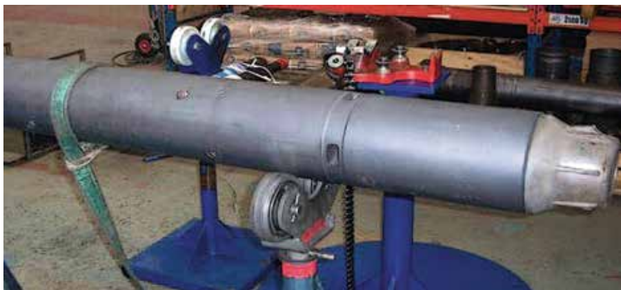
Fig. 1 – RFID controlled, downhole circulating sub for well clean-up, which was used in the North Sea by operator CNR
