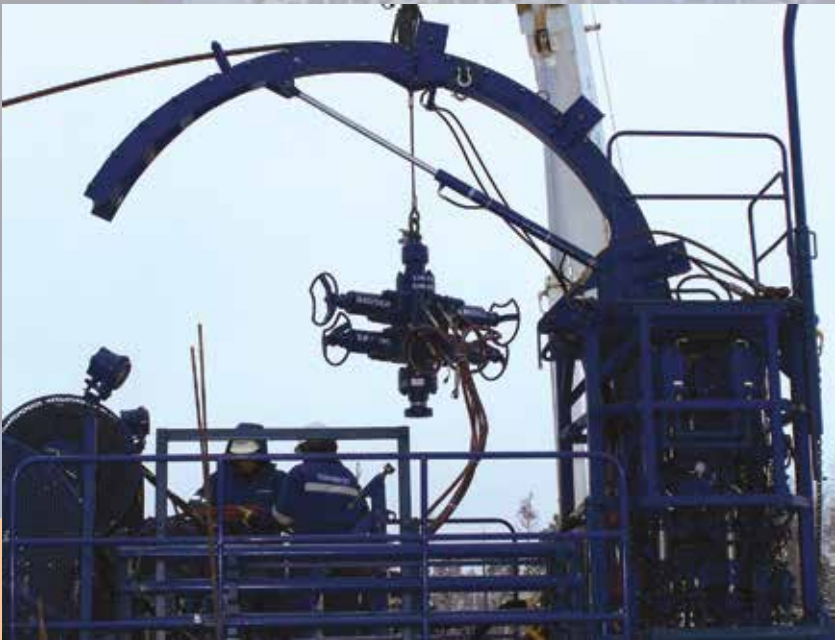
Pictures: injector with 27 ton lifting capacity on the test bench
