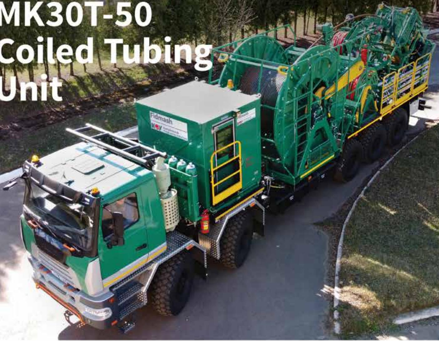
The Fidmash™ MK30T (MK30T-50) coiled tubing unit (CTU) is mounted on an 10x10 all-wheel drive chassis and represents a complete set of equipment for coiled tubing operations. Dressed for 1.75 in., this unit can run coiled tubing up to 2 in. in diameter. Air-conditioned cabins and fully winterized design.
